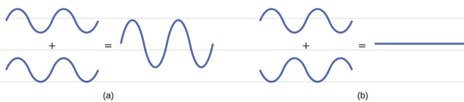
Figure 8.28 (a) When in-phase waves combine, constructive interference produces a wave with greater amplitude. (b) When out-of-phase waves combine, destructive interference produces a wave with less (or no) amplitude.
